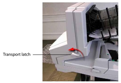
Figure 20: Opening the transport stacker cover
