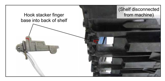
Rotate the front of the stacker finger's body up and gently squeeze the rounded
