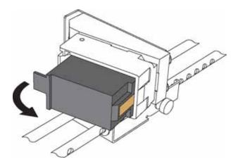
2 Insert the new cartridge by tipping the front end of the cartridge in first, and then pushing in the rear of the cartridge until it "clicks" into place.
