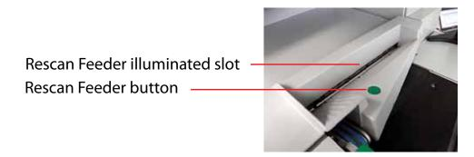
The Rescan Feeder can only be activated via the Rescan Feeder button when the machine is in a jammed or paused state.
