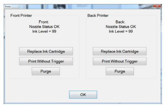
The Printer Information window provides access to printer maintenance features.
