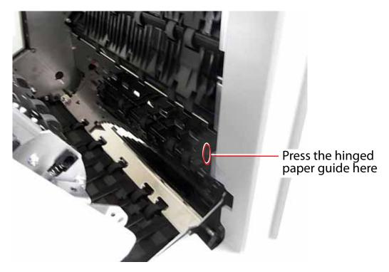
**b.** Swing open the paper guide to expose the printer assembly.
