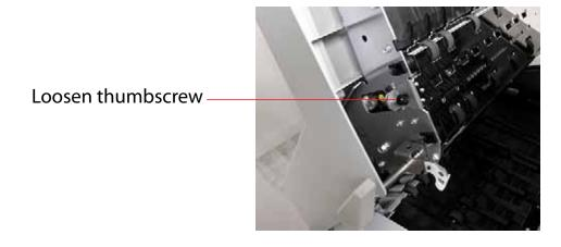
**b.** Swing open the paper guide to expose the printer assembly.
