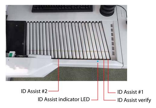
Figure 18: IDAssist sensors
